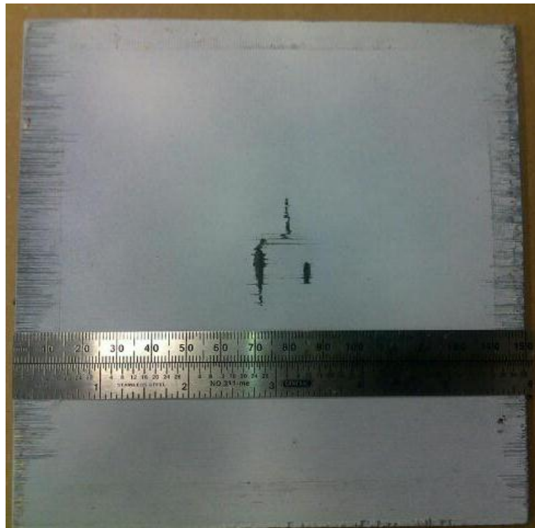
Figure 3.23: Visible Damage on the Back Side of Sample 48
